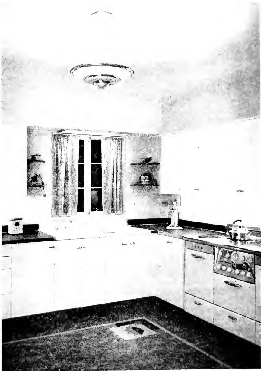
Good lighting in the kitchen is essential. General lighting is provided by the ceiling fixture, and every working surface is illuminated by built in lighting fixtures. Note the panel above the sink.
